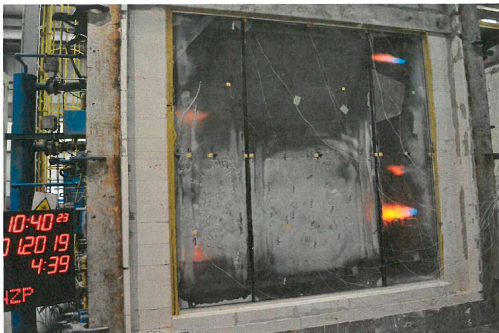
Photo 3. View of the heated surface of the test element in the 5th minute of the test
