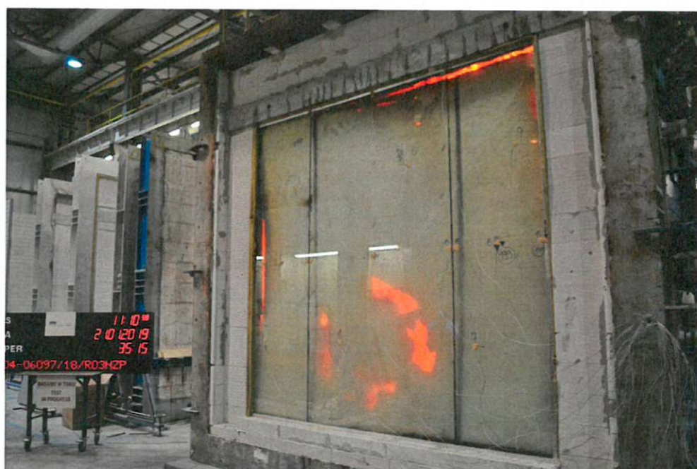
Photo 6. View of the non-heated surface of the test element at 36 minutes of the test
