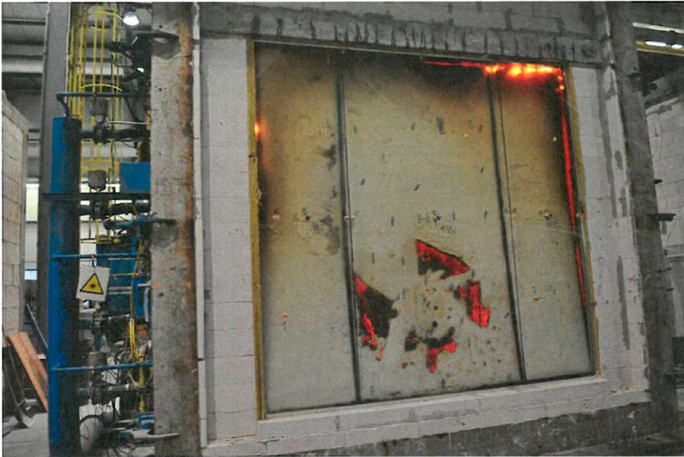
Photo 7. View of the non-heated surface of the test element after the test
