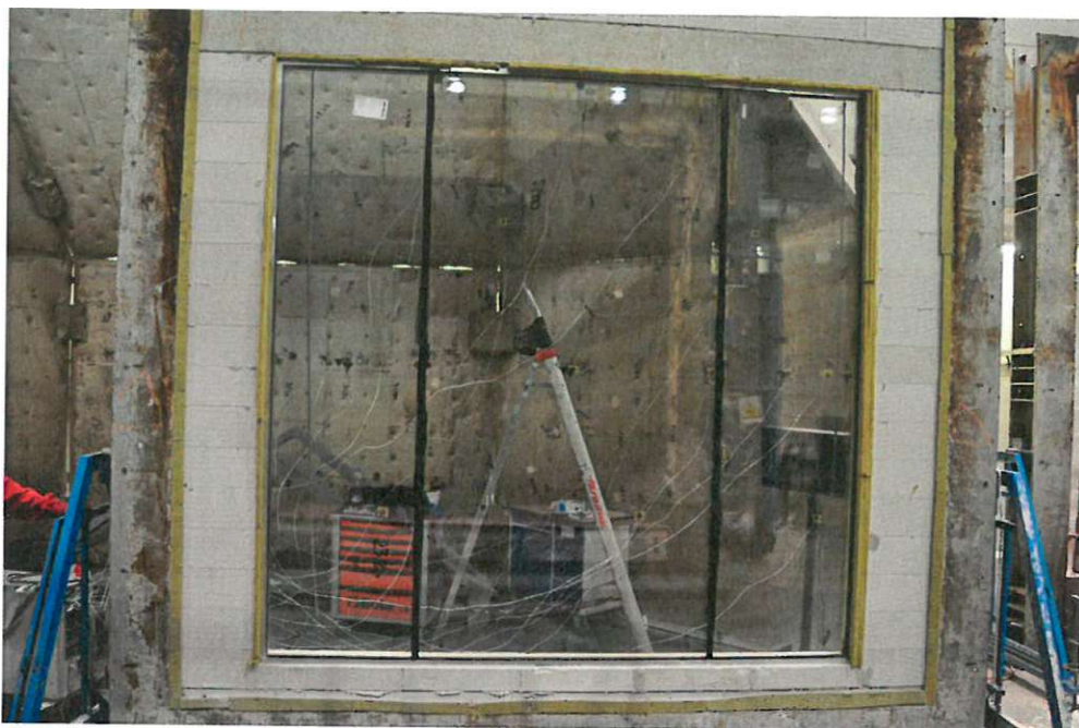
Photo 1. View of the non-heated surface of the test element before testing
