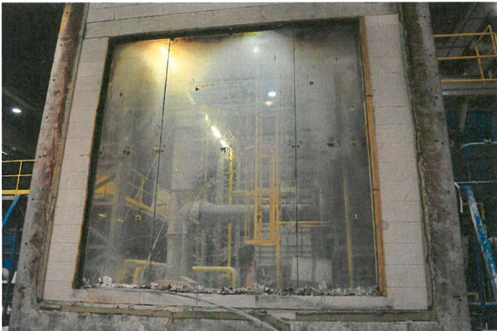
Photo 8. View of the non-heated surface of the test element after the test
