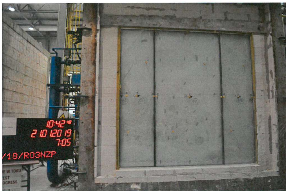
Photo 4. View of the non-heated surface of the test element at 7 minutes of the test
