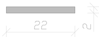
Figure no. 28: (KH0410) – ceramic gasket
