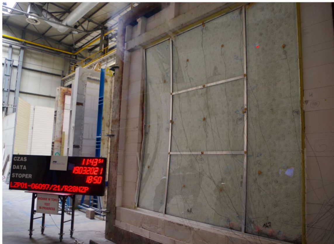
Photo 3. View of the non-heated surface of the test element at 19 minutes of the test
