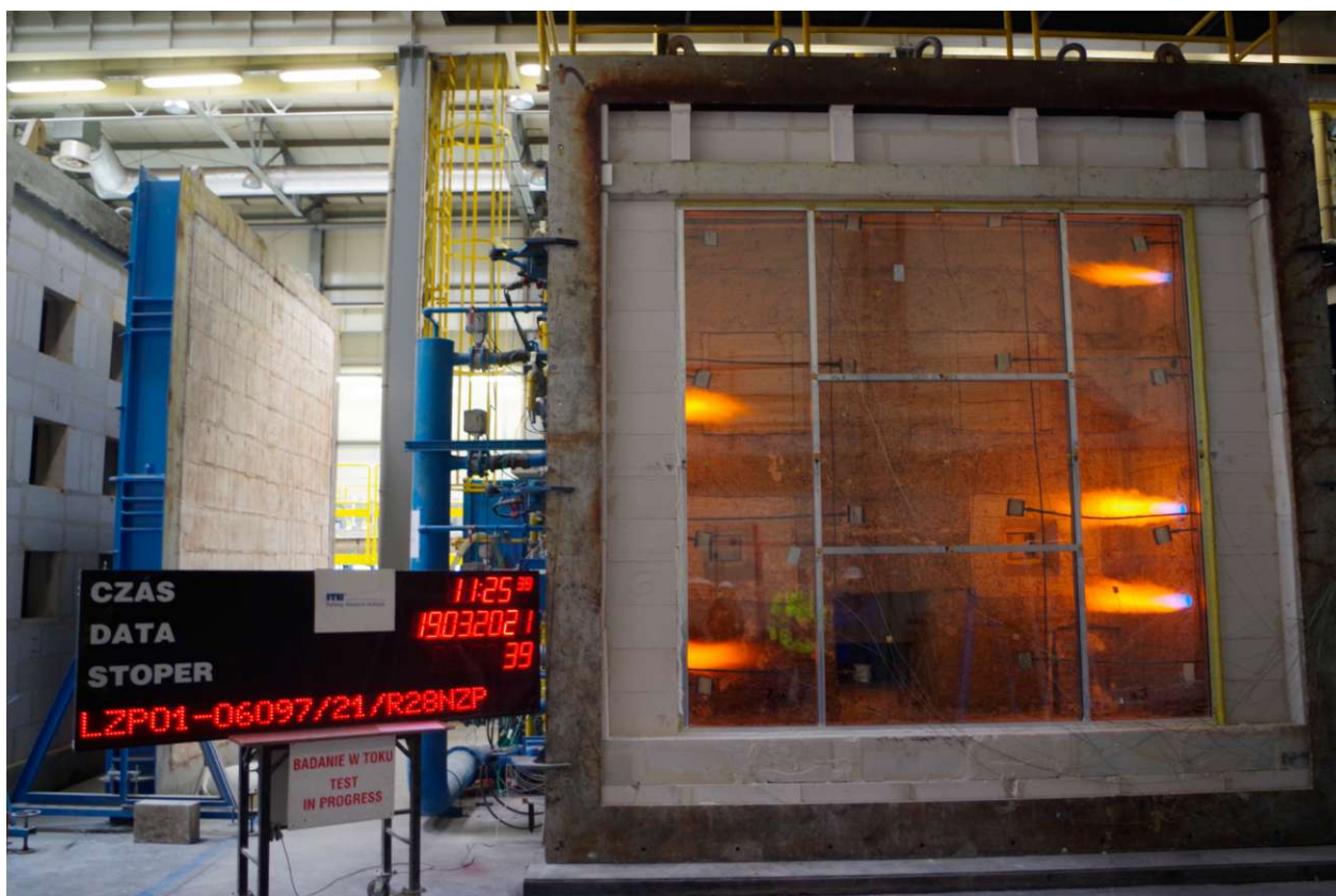
Photo 3. View of the non-heated surface of the test element at 1 minutes of the test
