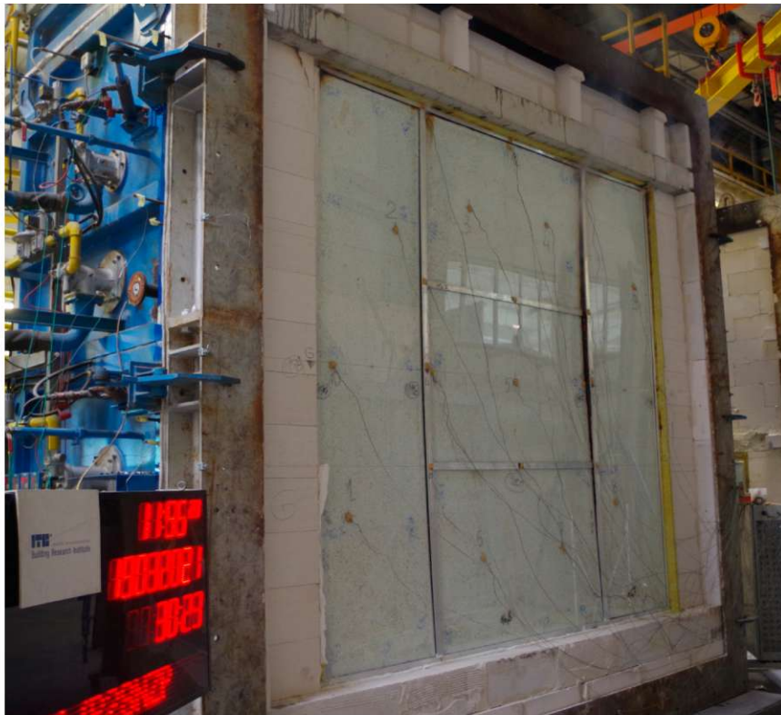
Photo 5. View of the non-heated surface of the test element at 31 minutes of the test
