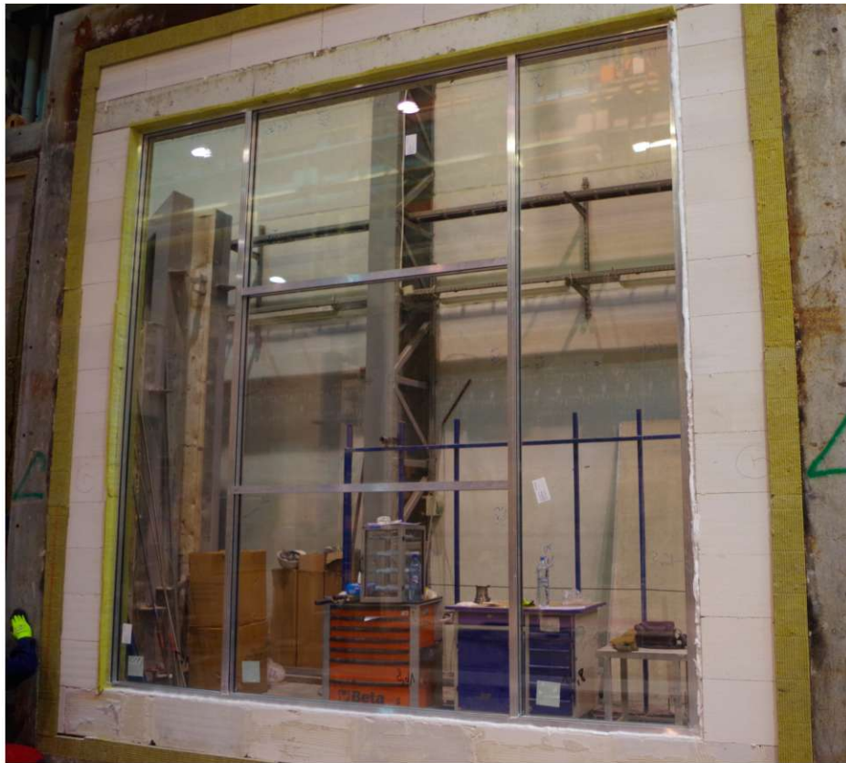
Photo 1. View of the non-heated surface of the test element before testing
