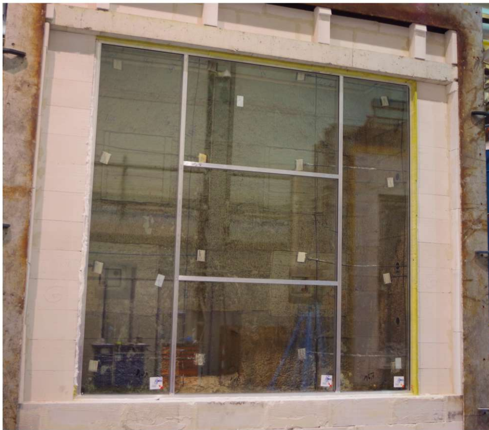
Photo 2. View of the non-heated surface of the test element before testing
