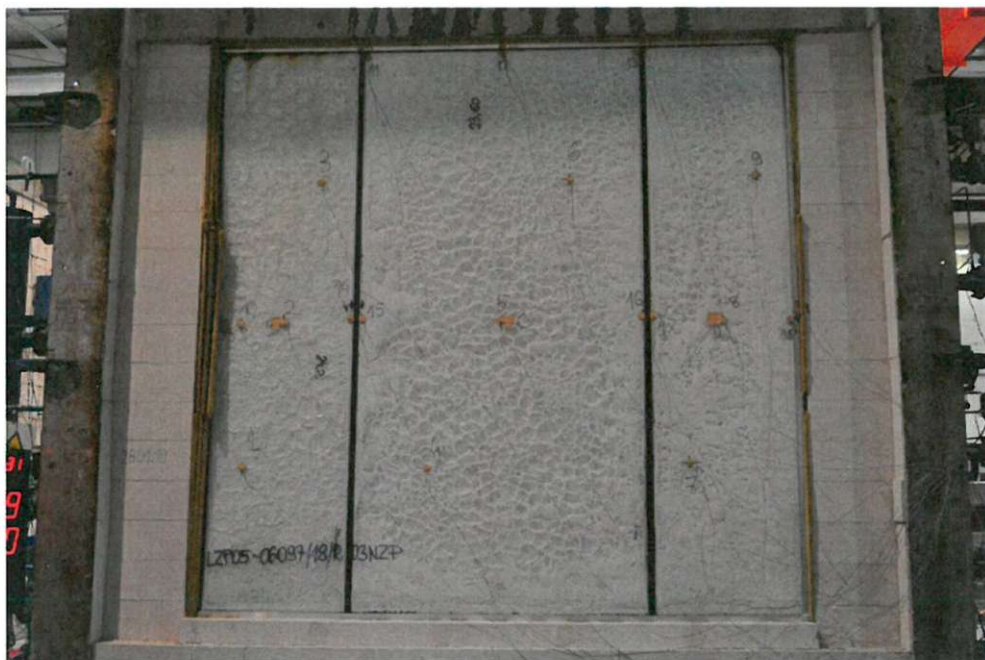
Photo 6. View of the non-heated surface of the test element after testing
