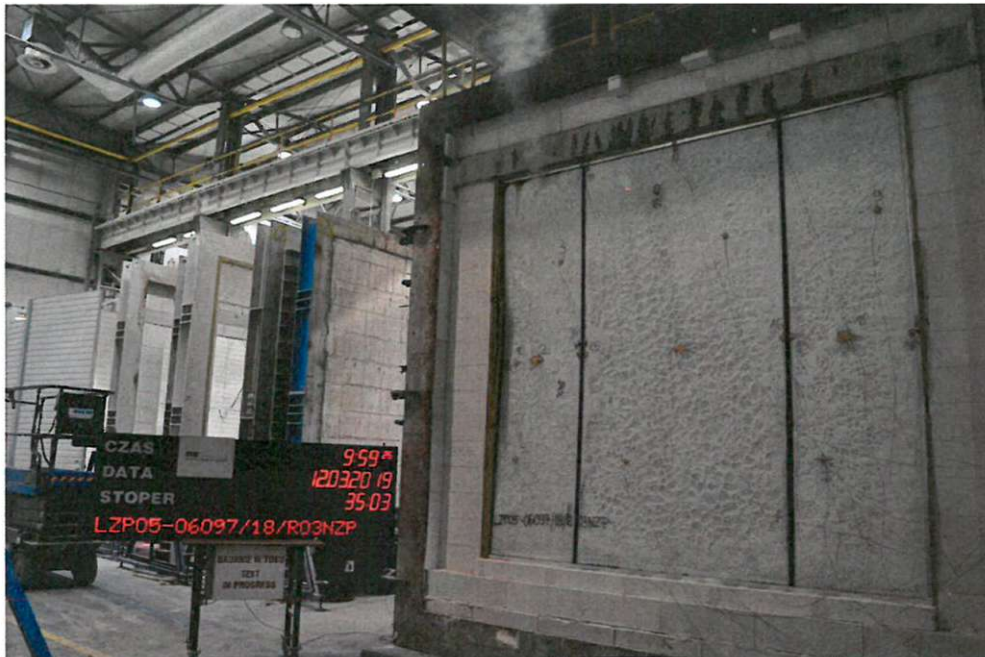
Photo 5. View of the non-heated surface of the test element at 36 minutes of the test
