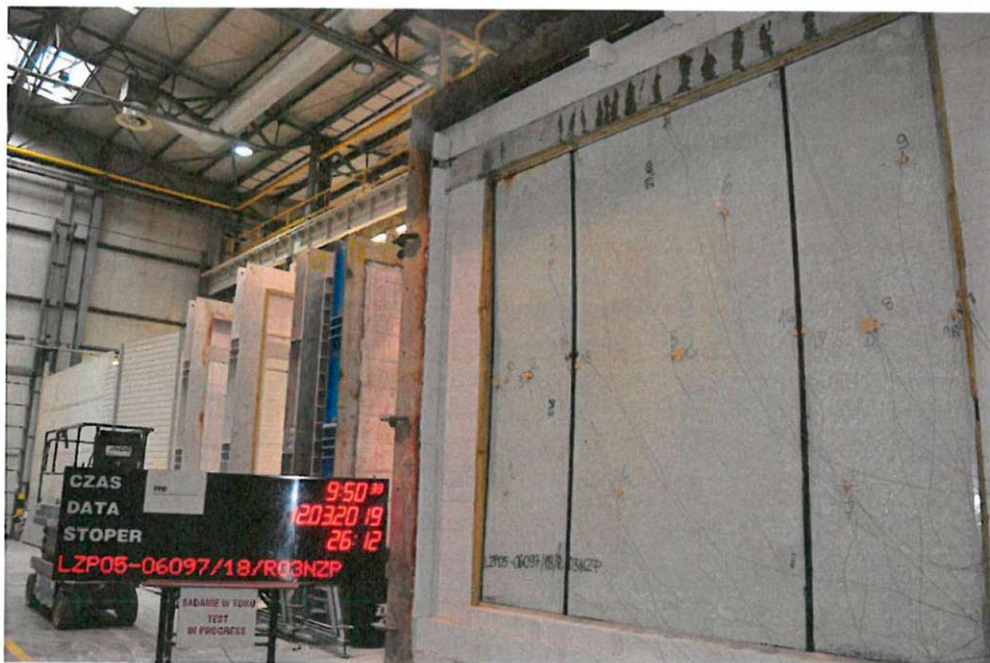
Photo 2. View of the non-heated surface of the test element at 27 minutes of testing
