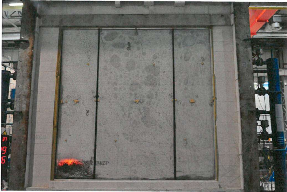
Photo 3. View of the non-heated surface of the test element at 11 minutes of the test
