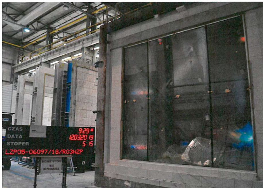
Photo 2. View of the non-heated surface of the test element at 6 minutes of testing
