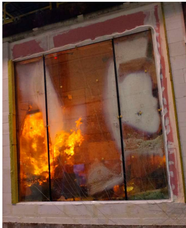
Fig. 2B. Unheated side of the test element, t = 8'10''
