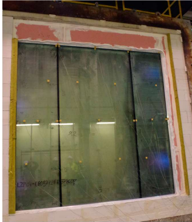
Fig. 1B. The unheated side of the test element before testing
