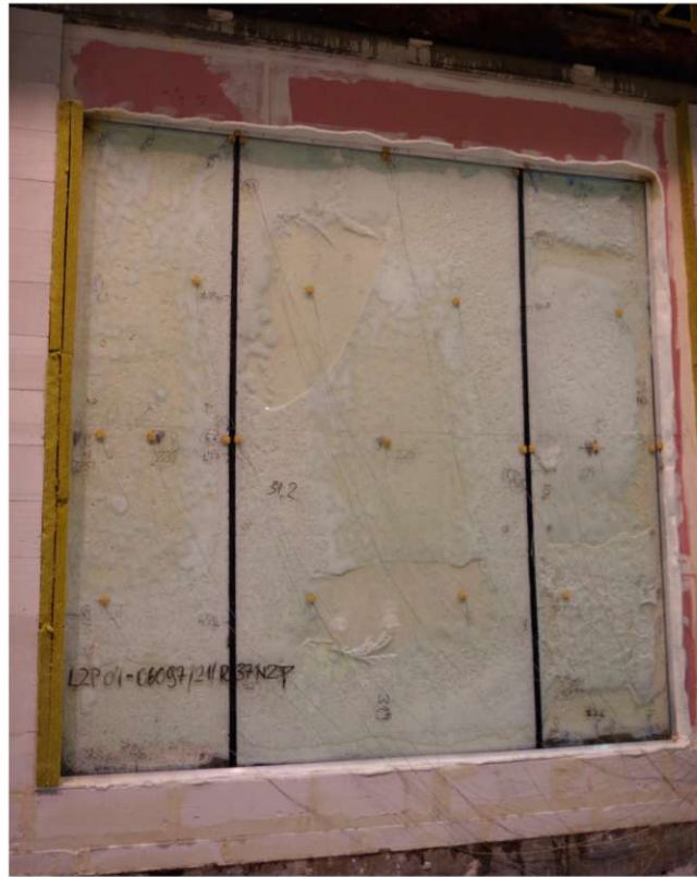
Fig. 3B. Unheated side of the test element, t = 31'20''
