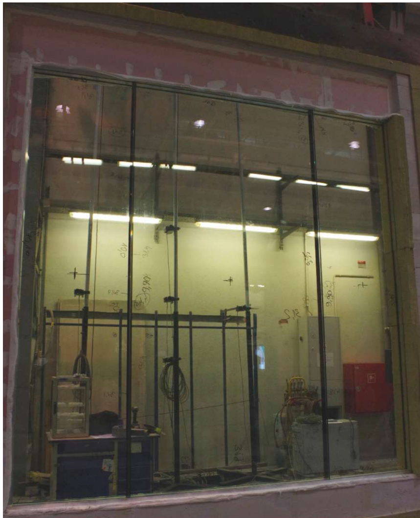
Fig. 1. Test element before testing - heated side
