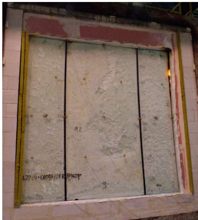
Fig. 6B. The unheated side of the test element after testing
