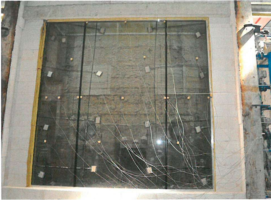
Photo 1. View of the non-heated surface of the test element before testing
