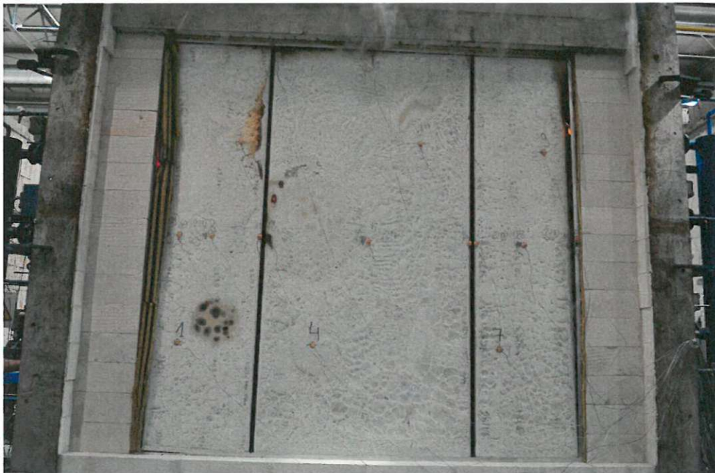
Photo 6. View of the non-heated surface of the test element after the test
