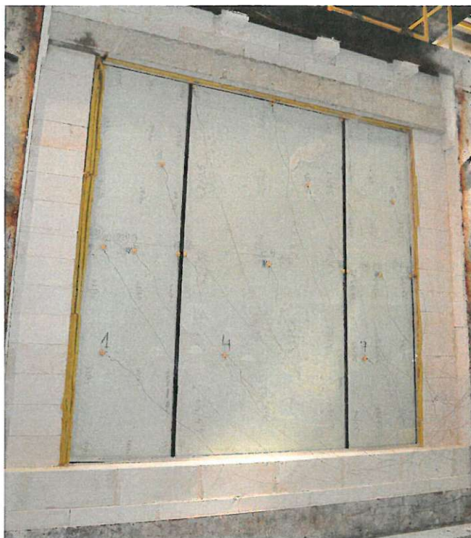
Photo 3. View of the non-heated surface of the test element at 16 minutes of the test
