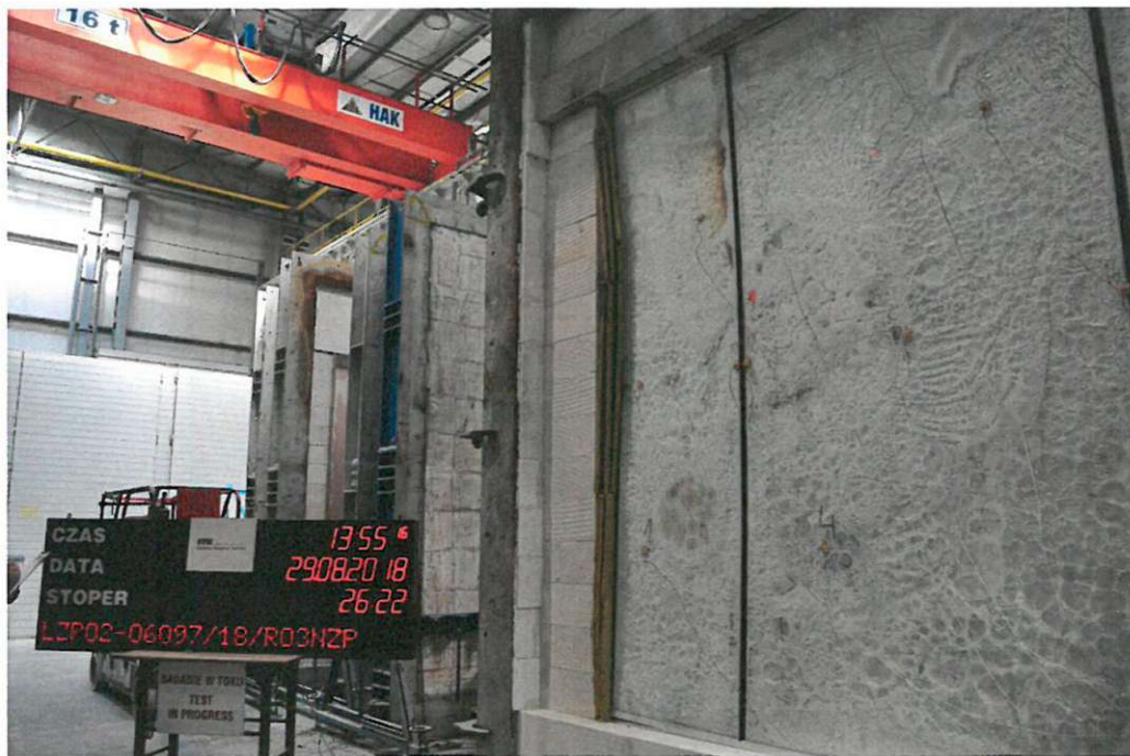
Photo 5. View of the portion of the test element unheated surface in the 27th minute of the test
