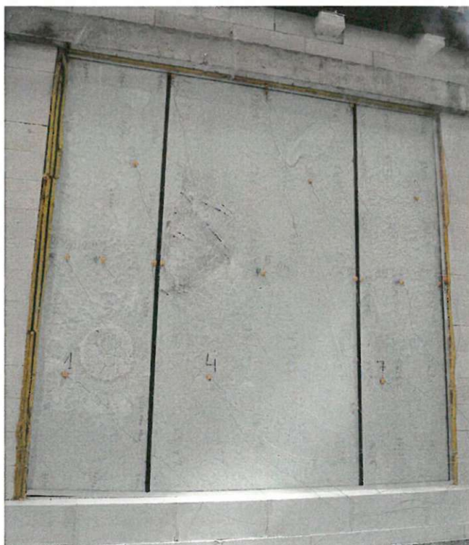
Photo 4. View of the non-heated surface of the test element at 21 minutes of the test
