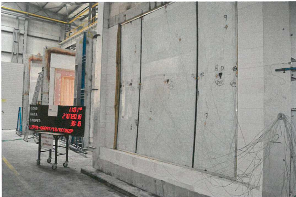
Photo 3. View of the non-heated surface of the test element at 31 minutes of the test
