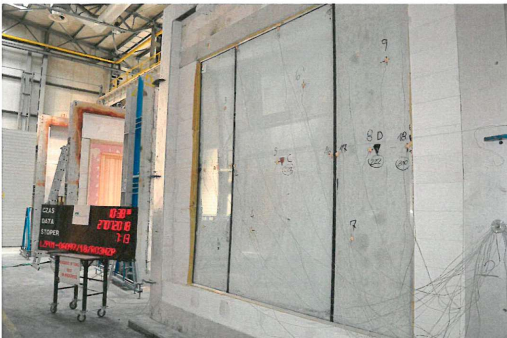
Photo 2. View of the heated surface of the test element in the 8th minute of the test
